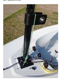
Step 2, Gooseneck locking lever on port side, it won't then interfere with outhaul
