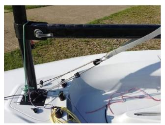
Step 4, Outhaul through outhaul line floating block and tie off with bowline around mast
